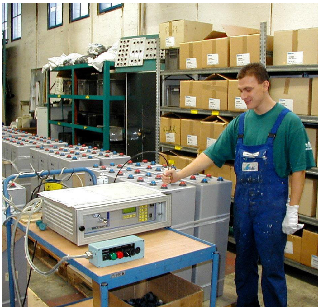
Figure 32 – Measurement of tightness with over pressure.
