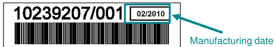
Fig. 1: Cell/Block Barcode example
