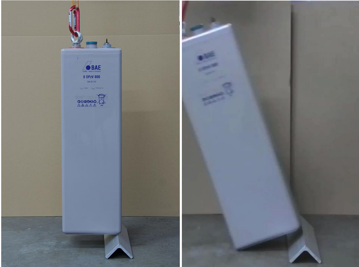
Figure 28 – Test set-up for the drop on the shortest edge.
