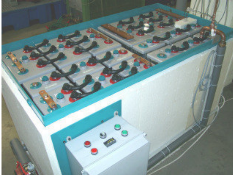
fig. a: Test equipment for the ageing at 62,8°C, laboratory BAE
