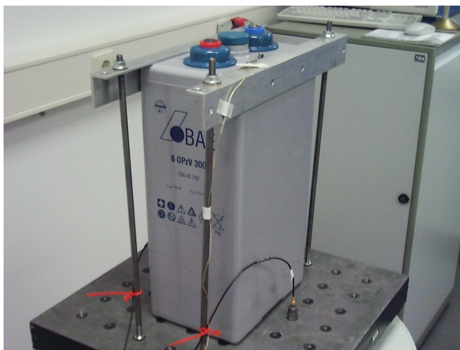
Figure 14 – Mechanical test on 2 V 6 OPzV 300 – Z axis.
