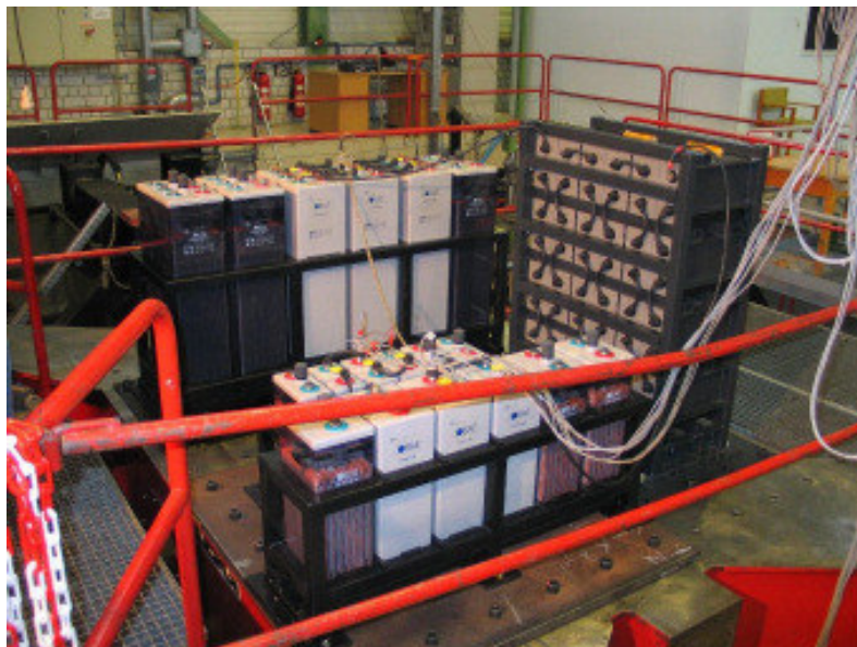
fig b: Test-batteries OPzV during the seismic test at IABG, Munich
