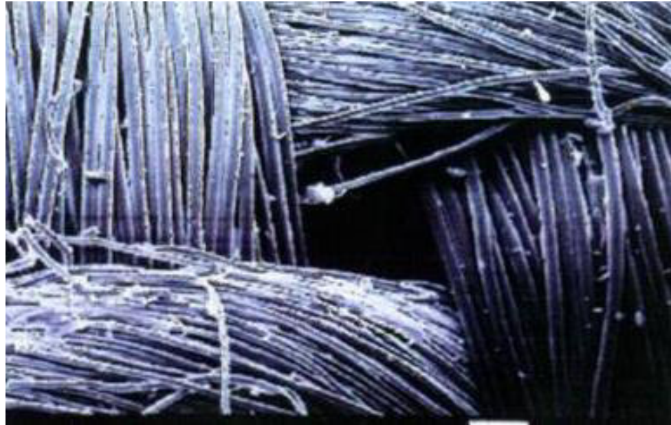
Fig 11: SEM of the woven gauntlet tubular pocket
