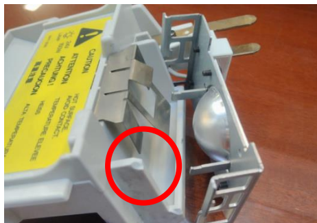
SOCKET LAMP AVERIADA
