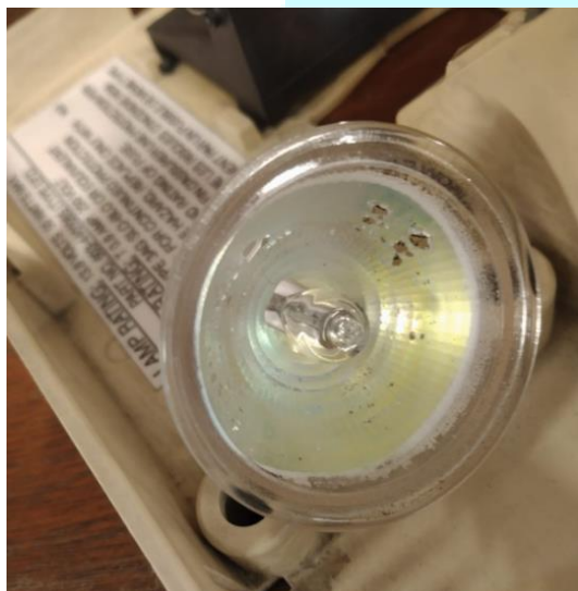
HALOGEN LAMP AVERIADA
