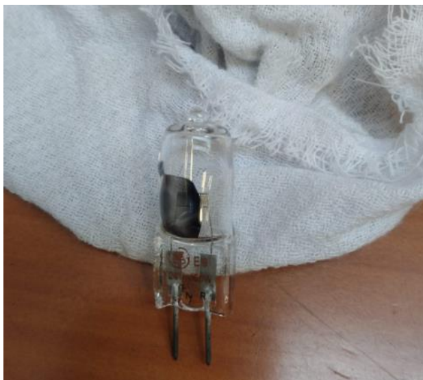
HALOGEN LAMP AVERIADA
