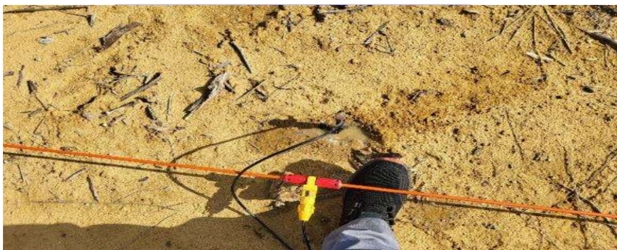
Figura 1 - 19 Conector Jumper, electrodo a take-out de cable multiconductor
