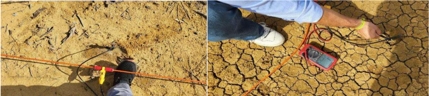
Figura 1 - 16 Conector Jumper, electrodo a take-out de cable multiconductor
